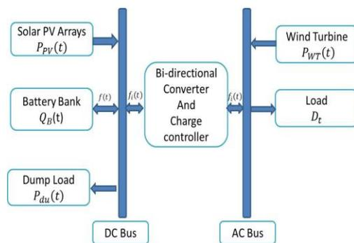
Fig. Schematic of renewable energy based isolated power system
