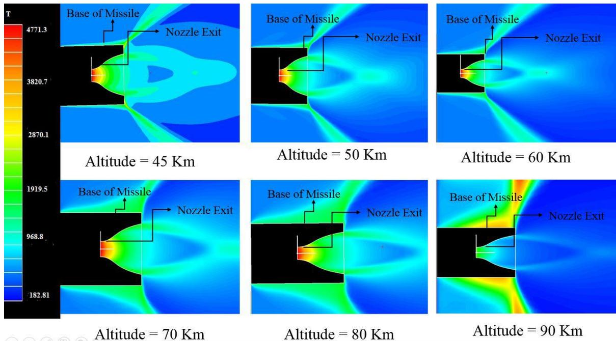
Fig: Temperature profile near the base of missile at different altitudes
